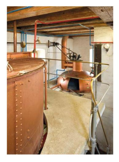
(left) Back to the future: The oldest brewhouse supplied by schulz and still in active service was built in 1844. And because it is wood fired, it complies with modern carbon-neutral standards. schulz is forging the way ahead with technology developed in house for carbon-neutral brewing, e.g. using biomass biomasse as a fuel
